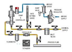
**Standard Pneumatic Controller Configuration**
