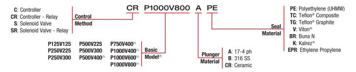
NOTE: (1) The 400, 600 and 800 motor cylinders are only available with the CR (controller-relay) or SR (solenoid-relay) control methods.
