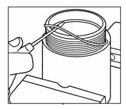
9. Remove the oiler body O-ring and pump/oiler connector nipple from the oil chamber. (Fig.62 & 63)
