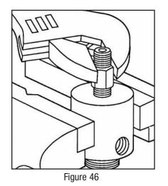
8. Use the same wrench to remove the bleeder plug from the fluid cylinder. (Fig.47)
