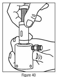
3. Remove the piston plunger assembly and motor return spring, and then remove the piston U-cup from the piston. (Fig.41 & 42)
