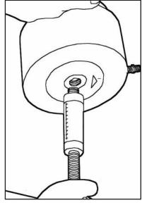
3. For all pumps except the P1500W400, remove the piston plunger assembly and the two O-rings. For the 1500W400 pump, remove two U-cups instead of the O-rings in this step. (Fig.55)
