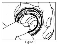
To reassemble the controller, reverse the above procedure. Be sure to replace all rubber components. Flare the U-cup out with your finger before installing the spool and apply a small amount of silicone grease (GS102149) to the U-cups and the upper/lower body inside diameter.
